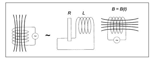
The setup is shown schematically above. The coil can be considered as an ideal coil in series with a resistance. The coil is imposed to a forced oscillation from an external field according to the voltage equation.
