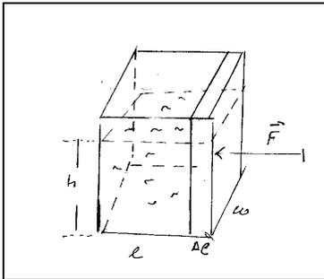
To simplify matters, we shall first look at a rectangular container with water, where the upper lid is open, and where one of the sides acts as a piston that can be moved in or out due to a force acting perpendicular to that side.
