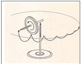
The figure shows such a gadget, where the massive wheel initially is put into rapid rotation and the axis is balanced vertically. If you let go the support in the free end, you would normally expect that the gyro would fall down, as would be the case, without the rotating disc.
