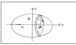
The volume of the ellipsoid can be found by by slicing it up in discs with radius y and thickness dx. The equation of the ellipse in the coordinate system
