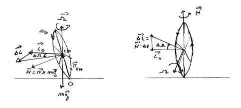
When you drive a bike the rotating wheels have an angular momentum, where its direction together with the spinning direction forms a right hand screw.
