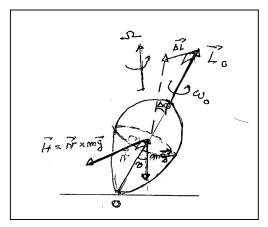
The direction of  $\Delta \vec{L} = \vec{H} \Delta t$ , is the same as in the example with the gyroscope, and conversely to what you might think, the constant angular momentum  $\vec{L}_0$  will get a horizontal twist  $\Delta \varphi$  in the positive circular direction, where:
