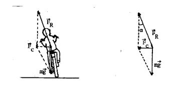
The cyclist is influenced by gravity  $\vec{F}_T$  and a reaction force  $\vec{F}_R$  from the ground. If the turn has constant radius and is traversed with constant speed v, the cyclist is performing a uniform circular motion with speed v and radius r. The vector sum of  $\vec{F}_T$  and  $\vec{F}_R$  then deliver the centripetal force  $\vec{F}_c$  necessary to uphold the circular motion.
