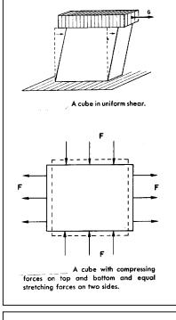
Next we shall see what happens, when we put a "shear" stress on a bulk of matter. By a shear strain, we mean the kind of distortion show in the figure to the left. For simplicity, let us look at the strains in a cube of material subjected to the forces, as shown in the bottom figure to the left. Again we shall break it up in two parts: The vertical pushes and the horizontal pulls. Calling the area of the cube face for A, we have for the change in the horizontal length.
