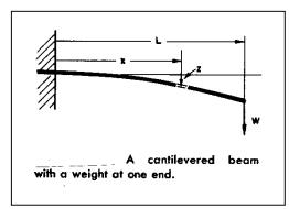
As another example of the beam equation (6.3), we shall find the deflection of a beam which is fixed in one end, with a force F (in the figure W) acting in the free end. We are interested in what the shape of the beam may be. The mathematical formula for the curvature in a point of z = z(x) is:
