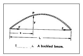
Consider the situation sketched above to the right in which a rod that normally is straight, is held in its bent shape by two opposite forces that push on the ends of the rod. Our aim is then to find the shape of the buckled rod and the magnitude of the forces at the ends.
