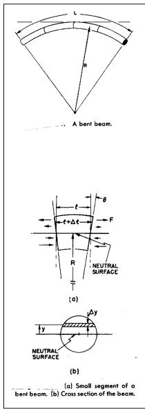
Now we shall look into bending of a rod or a beam, which is another matter concerning elasticity. (See the figure to the left). We shall first analyze which forces act on a cross section of the bar.
