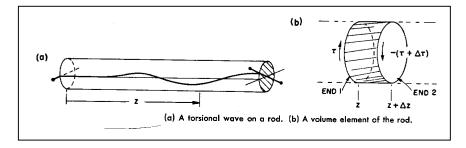
Let z be the distance to some point down the rod. For a static torsion the torque is the same everywhere along the rod and proportional to  $\phi/L$ , the total torsion angle over the total length. What matters to the material is the local torsion strain, which is  $\partial \phi/\partial z$ , so when the torsion along the rod is not uniform, we should replace (4.4) by
