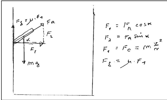
We shall then look at the situation, where a motorbike moves on the wall in a vertical cylinder, that is, driving the wall of death. First we shall assume that there is no friction between the wheels and the wall. The motorbike (only one wheel is drawn in the figure) is affected by gravity  $F_T$  and the reaction force  $F_R$  from the wall of the cylinder. The wheels are assumed to have an angle  $\alpha$  with horizontal.
