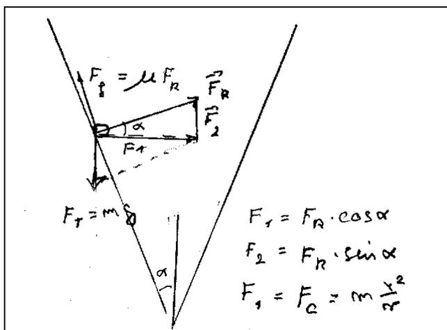
We shall consider a spherical bullet, which performs a circular rolling motion in a cone. Half the top angle of the cone is designated  $\alpha$ . First we shall assume that there are no friction between the bullet and the walls of the cone, and that the bullet performs a pure rolling.
