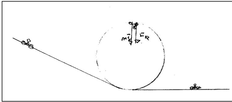
In the upper position the carriage is affected by gravity  $F_T = mg$  and the reaction force  $F_R$  from the rail. They both have the same direction downwards, and together they form the resulting force on the carriage. When a body perform a circular motion the resulting force is equal to the centripetal force  $F_c = F_T + F_R$ .
