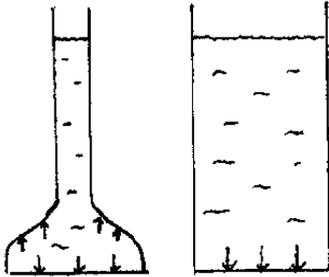
The two vessels, shown to the left, have the same ground surface, but different volumes. If they are filled with liquid to the same height, then according to the formula (2.2), the pressure at the two bottoms should be the same. Since the two bottom surfaces have the same area there should also be the same force on the bottom surface!
