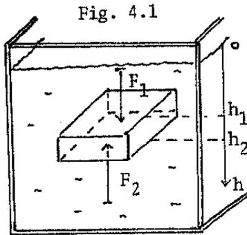
The figure shows a rectangular box immersed in a liquid having density  $\rho$ .
