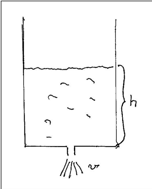
We shall consider a barrel filled with a non viscous liquid, having an outlet at the bottom.
