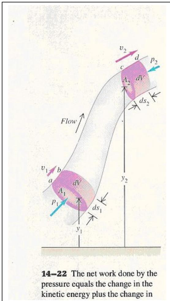
We shall now derive Bernoulli's law, which for a laminar i.e. non turbulent gives the relation between the pressure  $p$  and the streaming velocity  $v$ , at that point. Again we shall look at a tube, having the ends at (1) and (2).
