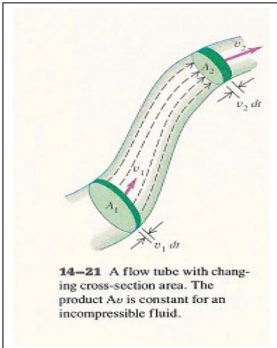
In the figure we have drawn a (mathematical) "tube", which follows a streamline. I might also be a physical tube, in which the liquid flows, but this is without importance).
