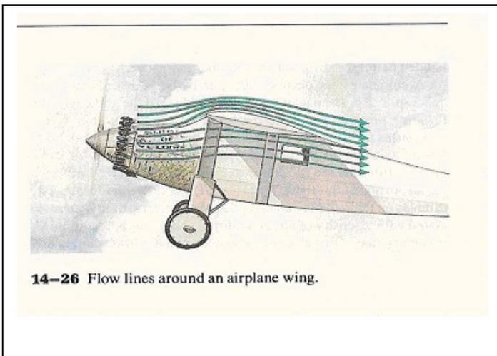
The figure demonstrates the principle of flying according to Bernoulli's law.
