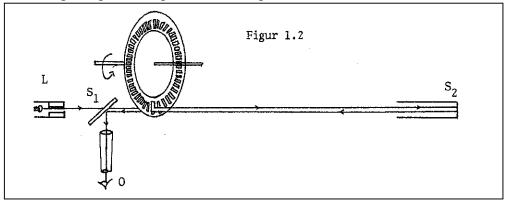
L represents the source of light, from which the light propagates through the semi transparent mirror  $S_I$ . The light then passes a rotating disc, equipped with a circular row of equidistant holes in a manner, so that the width of the hole is equal to the separation between them.
