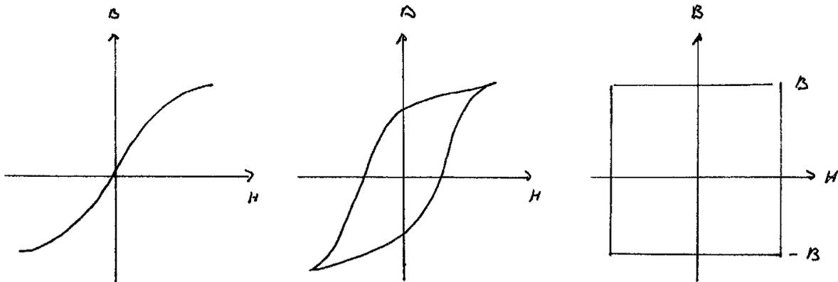
The potential energy of a magnetic moment is  $E_{pot} = \vec{\mu} \cdot \vec{B}$ , and we shall evaluate the loss in potential energy, when a magnetic moment is put through the curve, starting and ending in the same point.
