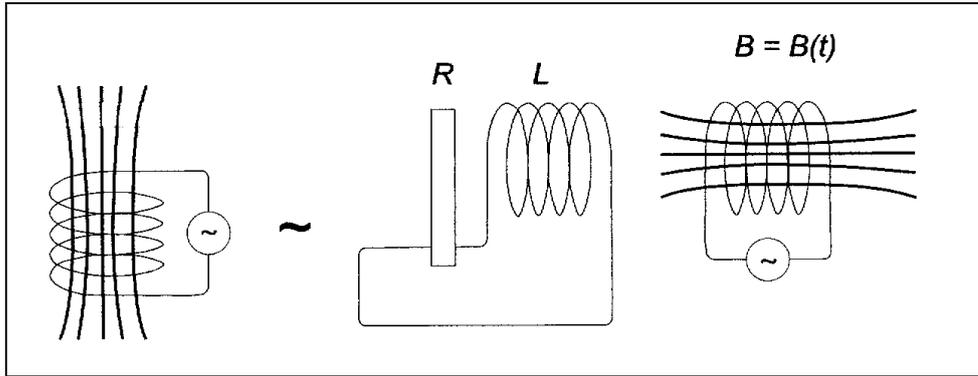
The setup is shown schematically above. The coil can be considered as an ideal coil in series with a resistance. The coil is imposed to a forced oscillation from an external field according to the voltage equation.
