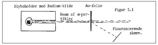
The alpha source is placed in a lead block, having a narrow pipe to secure a collimated stream of alpha particles. (Alpha particles are completely absorbed in less than one *mm Pb*.)
